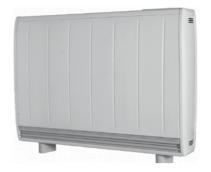
These are a more modern version of a storage heater. The heater will take charge during the night time off peak period and release the heat on demand during the day. There is a built in booster should the heat. run out, but this will not come on unless you manually activate it on the heater controls.
