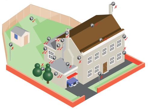
This illustration is for guidance only. It shows the possible positions of antennas.
